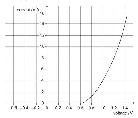
The diode is connected in series with a resistor and a  $6.0\,\mathrm{V}$  battery. The current in the circuit is  $8.0\,\mathrm{mA}$ .
